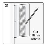
Wood Cutout: Remove middle section of flush pull template, position at desired backset and mark cutout outline. Use midline as height reference. Cut 16mm rebate
