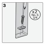
For wooden doors: install woodfix brackets at top and bottom of cutout on both sides of the door.
