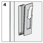
Insert offset flush pull into cavity. Push in and down so it grips onto the bottom bracket or edge.
