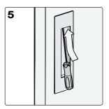
Use Mardeco hex tool to tighten grub screw inside top of offset flush pulls. Ensure they are fitted firmly.
